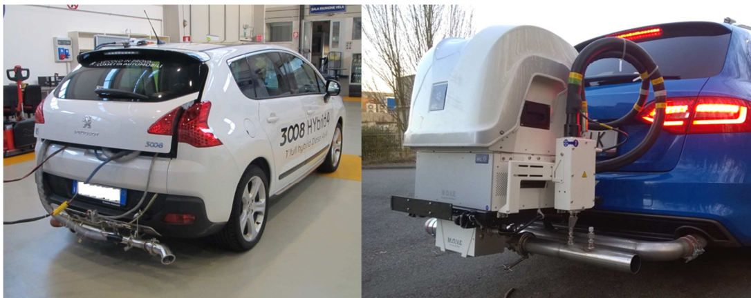
Figure 10. Routing heated probe left) from the inside of the vehicle; right) outside of the vehicle.
