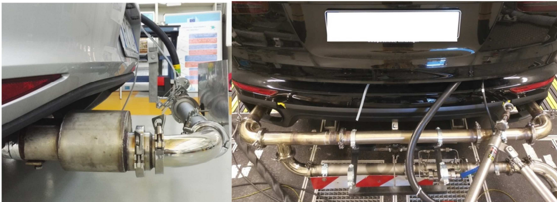
Figure 5. EFM Installation left) using a tailpipe adaptor; right) tubes and collars on a dual exhaust
