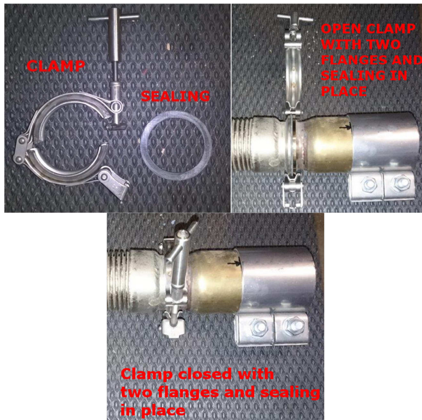
Figure 4. Installation of the EFM: elements for clamping
